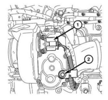
Remove the bolts (2, 3) and the turbocharger actuator (1).
