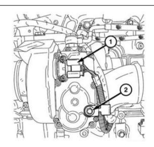
Now, after actuator is installed, using scan tool, perform the self-calibration portion of the "VG Turbocharger Actuator Pre-Alignment/Self Calibrate routine.
