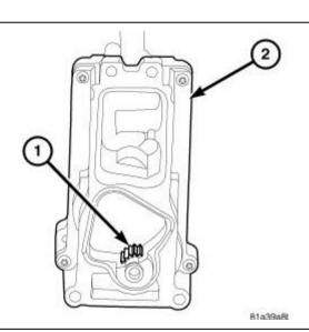
Connect turbocharger actuator wire harness connector. Connect both negative battery cables.
