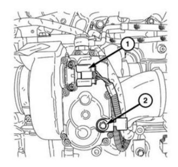
Disconnect the turbocharger actuator wire harness connector (1) from the turbocharger by cleaning the connector to remove debris, pulling the light gray release lever away from the locked position with your thumb nail until it clicks into the unlocked position, then holding the light grey release lever down while pulling the connector apart.
