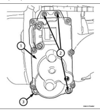
Using an Allen Wrench, tighten the remaining cap screw (3) until it is flush with the actuator body. After screw (3) has been brought flush with the actuator housing, tighten the screw an additional 90° turn.
